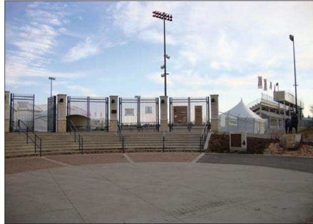
Plaza configuration, stairways, railings, and decorative wrought-iron fencing controls access into this large stadium.
