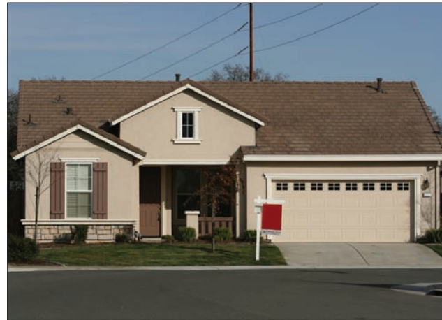
This home uses a grade change and lawn to demarcate the public street from the property line. The recessed porch vestibule further divides the space into a semi-private area prior to entering the private space inside the front doorway.
